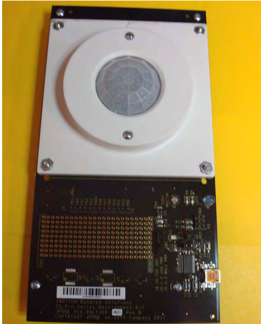
Figure 7. Assembled Circular 0.77" Lens Holder and Circular Lens Installed on the ZMOTION 20-Pin Development Board
