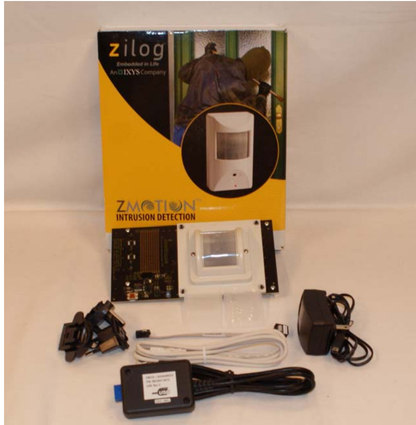
Figure 1. ZMOTION Intrusion Detection Development Kit Contents
