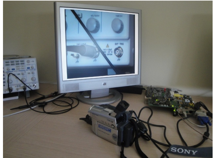
Figure 9: Photo of the deinterlacer bench setup
