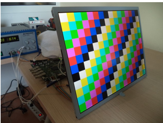
Figure 7: LVDS demo showing Sharp LCD 1280x800 test pattern display
